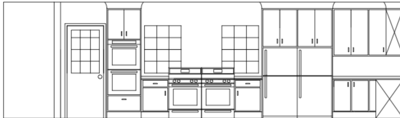
② ELEVATION OF KITCHEN WALL SCALE: \frac{3}{8}'' = 1'
